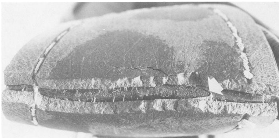
FIG. 2—View of crack in sole. Arrow indicates hole in moisture barrier.
